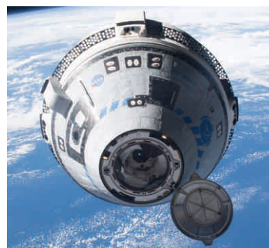
The Starliner approaching the ISS for docking. Its nose-cone and parachute compartment cover are open and we can see the docking system.
